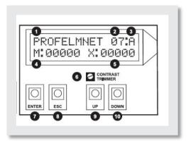
The 4033 has an LCD display through which the user can select all the settings and programming of the control board functions, easily and quickly. The user has the ability to customize the control board as they wish according to the conditions of their installation.
