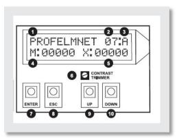
The 4114 has an LCD display through which the user can select all the settings and prog ramming of the control board functions, easily and quickly. The us er has the ability to customize the control board as they wish according to the conditi ons of their installation.
