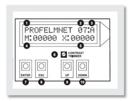
The 4050 has an LCD screen through which the user can select all the settings and programming of the control board functions, easily and quickly. The user has the ability to customize the control board as they wish according to the conditions of their installation.
